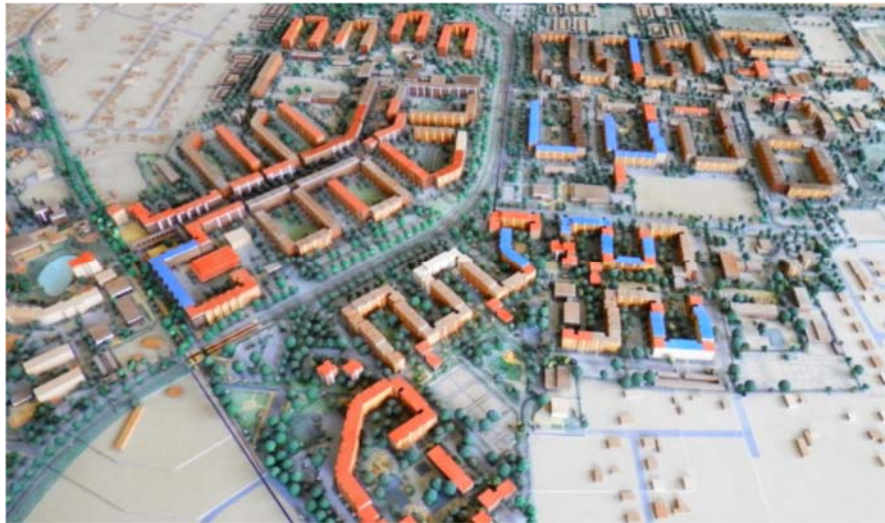
Figure 4. The “Neu Olvenstedt” Estate in Magdeburg - a model shows the process of planned demolition starting from 2002: buildings signed in red were demolished, of the marked with blue some upper floors were dismantled; (Author’s photo of a model, source [14]).
