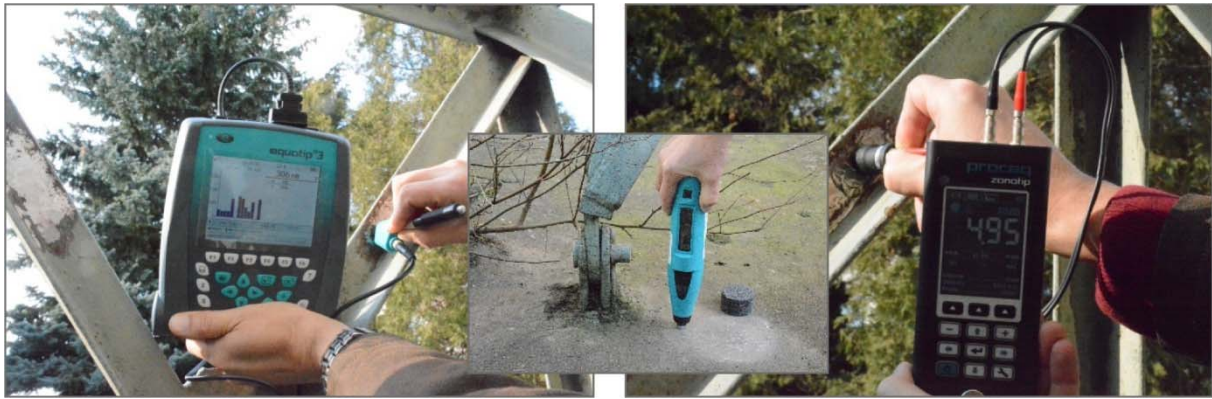
Figure 2. Documentation of non-destructive tests of steel and concrete carried out "in situ"
