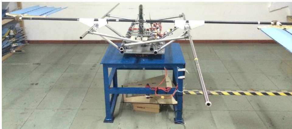
Figure 1. Rotary platform for force measurement.
