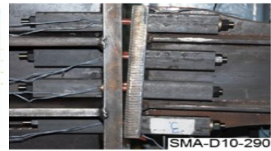
Figure 10. Detailed connection deformation ([37])
