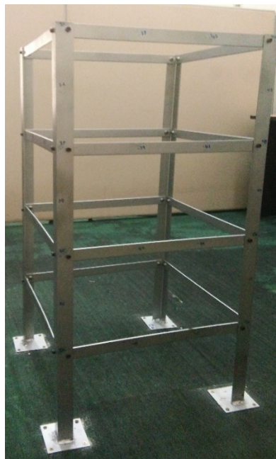
Figure 1. Frame structure with bolted joints.
