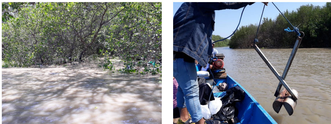
Figure 1. (a) station location in mangrove area (b) Sediments sampling using an Ekman grab.
