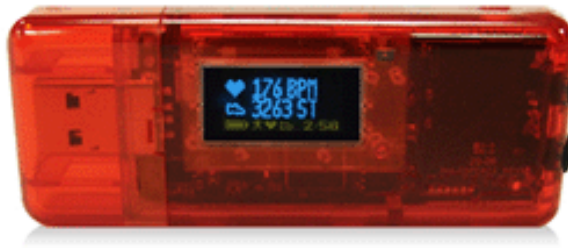
Figure 3: The Actigraph Actitrainer accelerometer device
