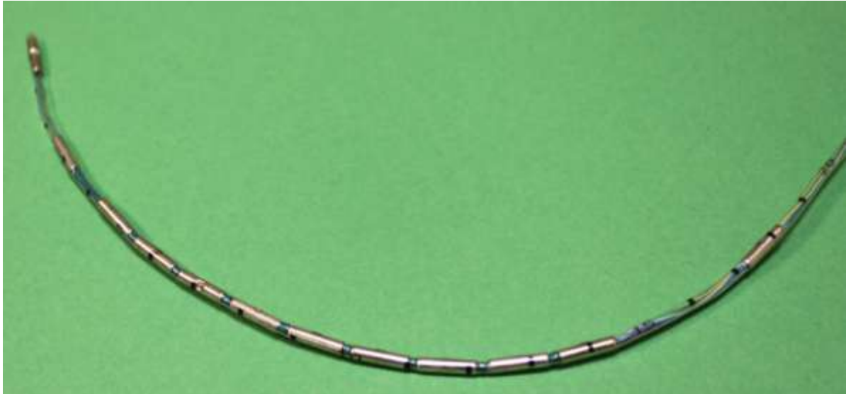
Figure 5.1. 12-sensor pH catheter
