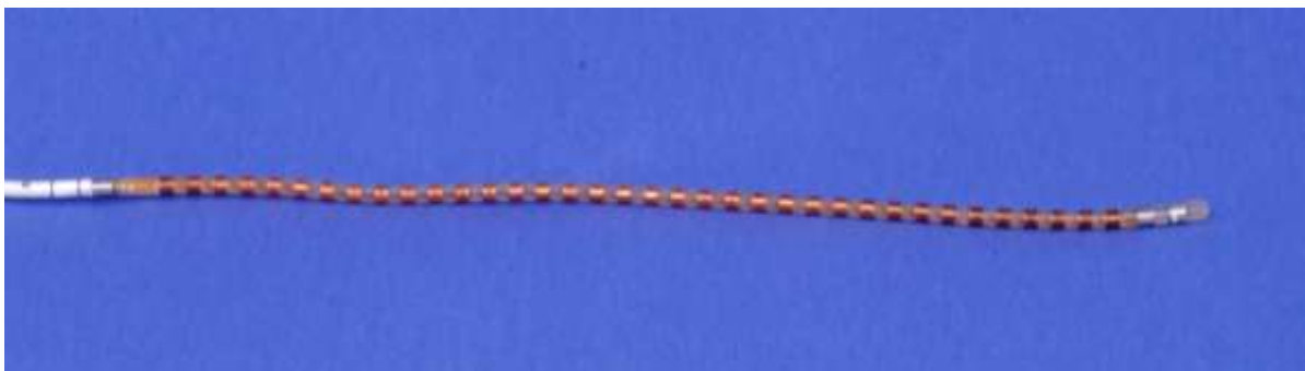
Figure 5.3. Manoscan® 36-sensor high-resolution manometer
