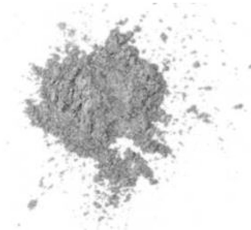
Figure 9. Base powder used in 3D implant creation
