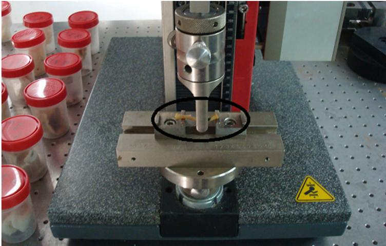
**Figure 1.** The three-point bending test on the tibia. The bearing span was 20 mm. The middle of the tibial osteotomy was set as the loading point with a loading speed of 1 mm/min. During the loading process, the loading direction was consistent and the specimens were kept wet.
