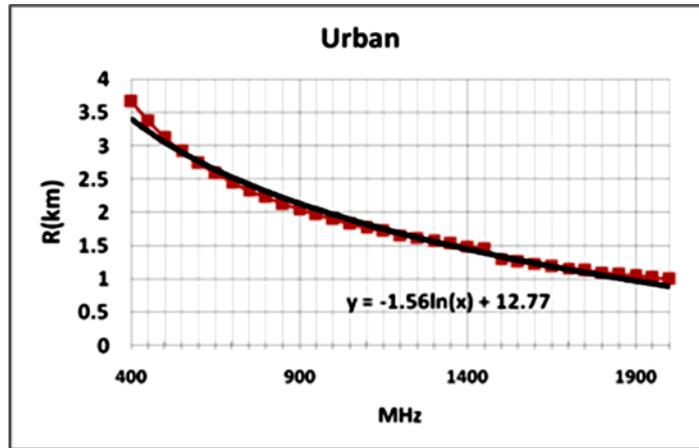
Figure 3 Frequency vs Range on band 400MHz -1900 MHz.
