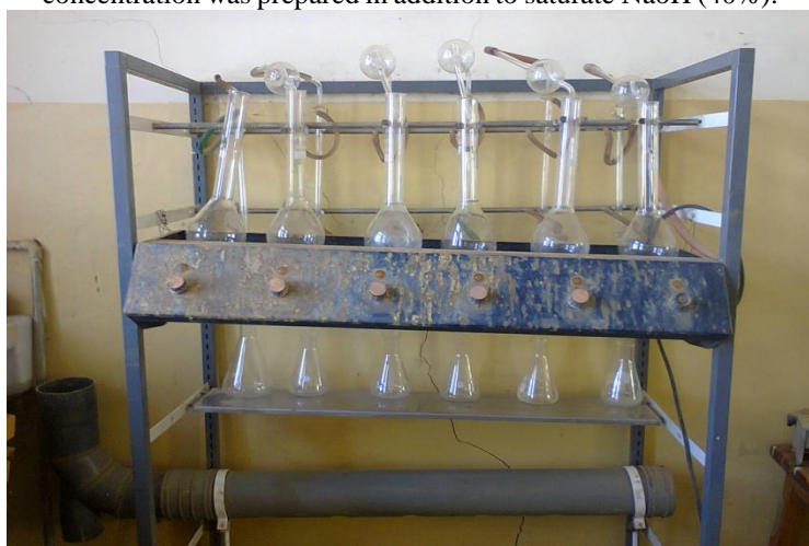
Figure 3. Kjeldahal apparatus used for protein digestion Distillation
