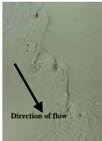
Figure 2 Vortices at the interface between the main channel and floodplain flow, Medicine Hat, Alberta (Tuitoeck, D.K., [2]).
