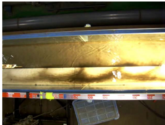
Figure 18 Experiment result of horizontal vortices.
