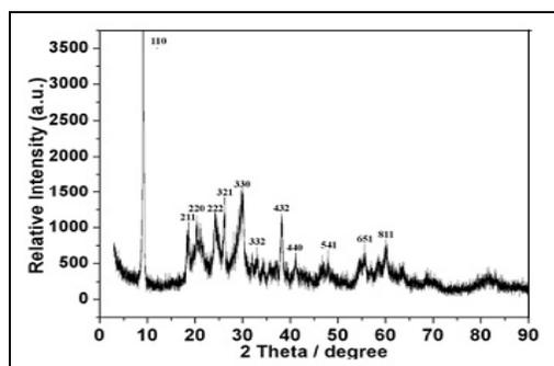
Fig. 1b. XRD patterns of AIPW catalyst
