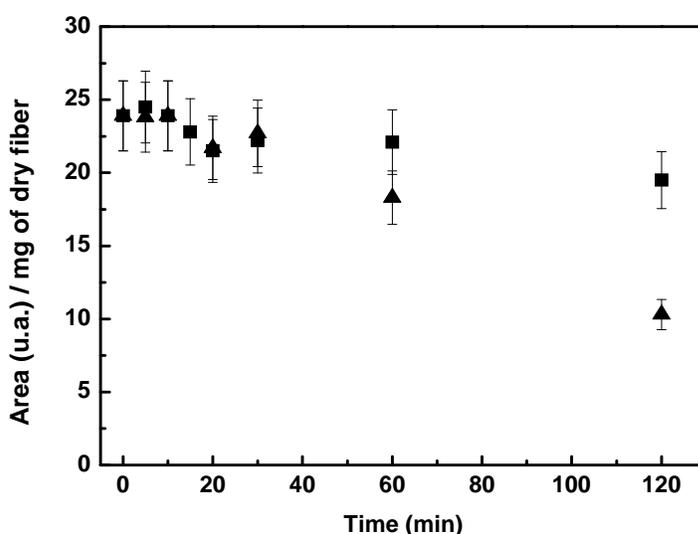
**Fig. 3.** Concentration of phenoxy radicals, reported as areas of the EPR resonances divided by the fiber weight, as a function of time for CTMP fibers in air (▲) and in argon (■).
