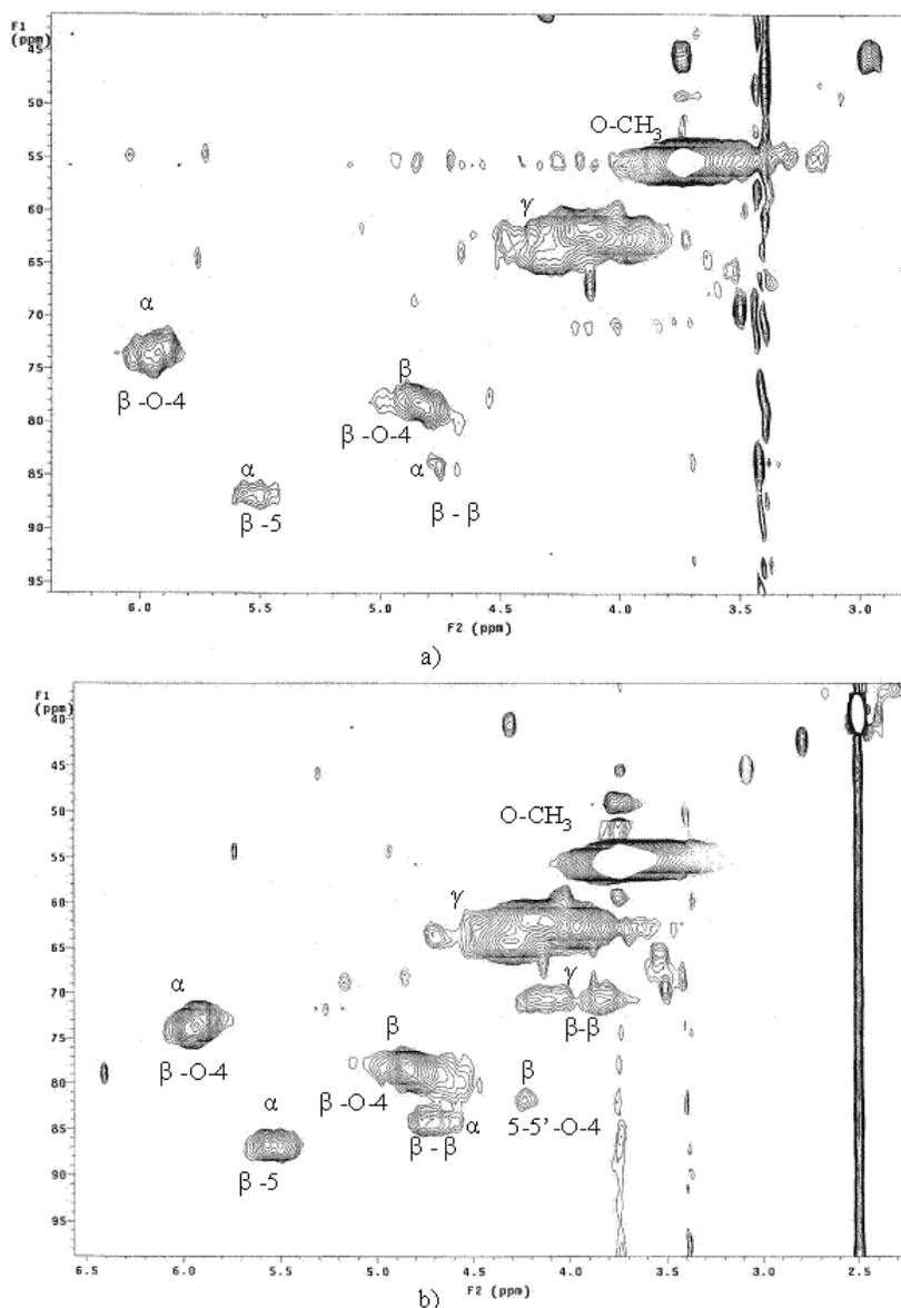
**Fig. 4.** 2D-HSQC spectra of acetylated lignin from CTMP fibers a) untreated and b) after plasma treatment (0.4 mbar Ar pressure, 75 W RF power and 2 pulses of 30 s).
