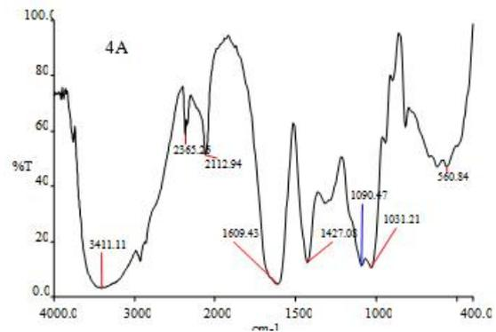
**Fig.4.** IR spectra of drug loaded beads
