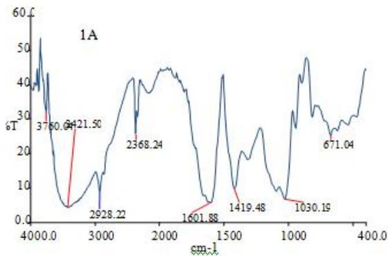
**Fig.1.** IR spectra of sodium alginate
