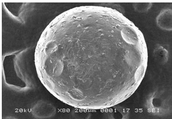
**Fig.5.** SEM photograph of drug loaded bead (A4) at 80 x
