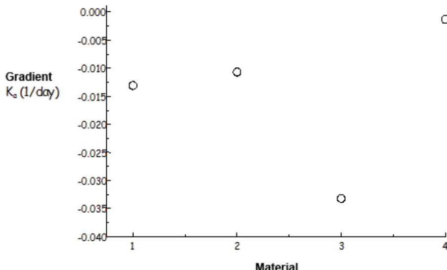
Figure 8. Gradient of change,  $K_a$ , for tested materials: 1) aqua ionobond; 2) ionoseal; 3) life; 4) cegal NV.
