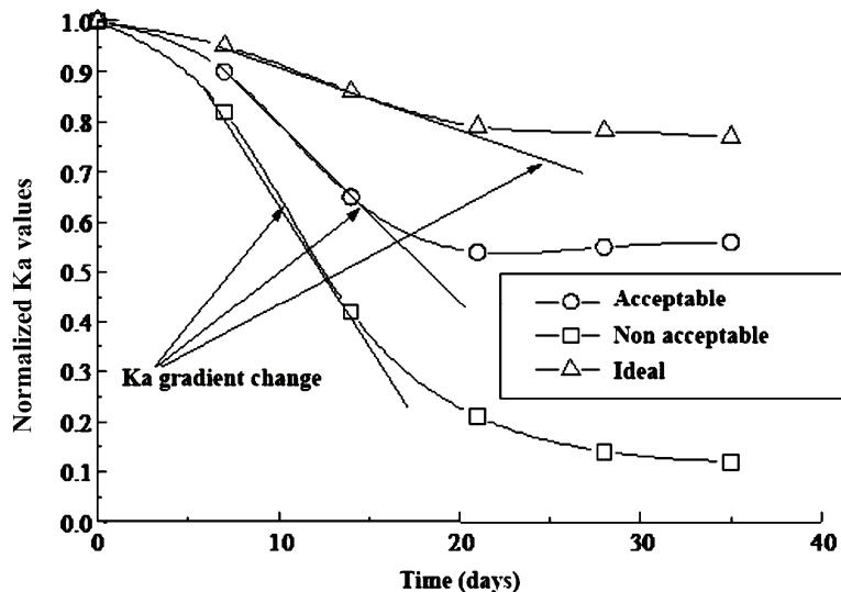
Figure 5. Hypothetical adhesion coefficient changes.
