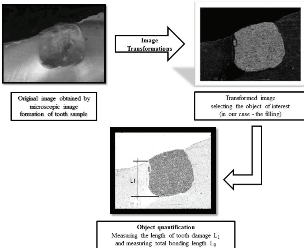
Figure 6. Steps of adhesion coefficient measurements ( $K_a = L_1/L_0$ ).
