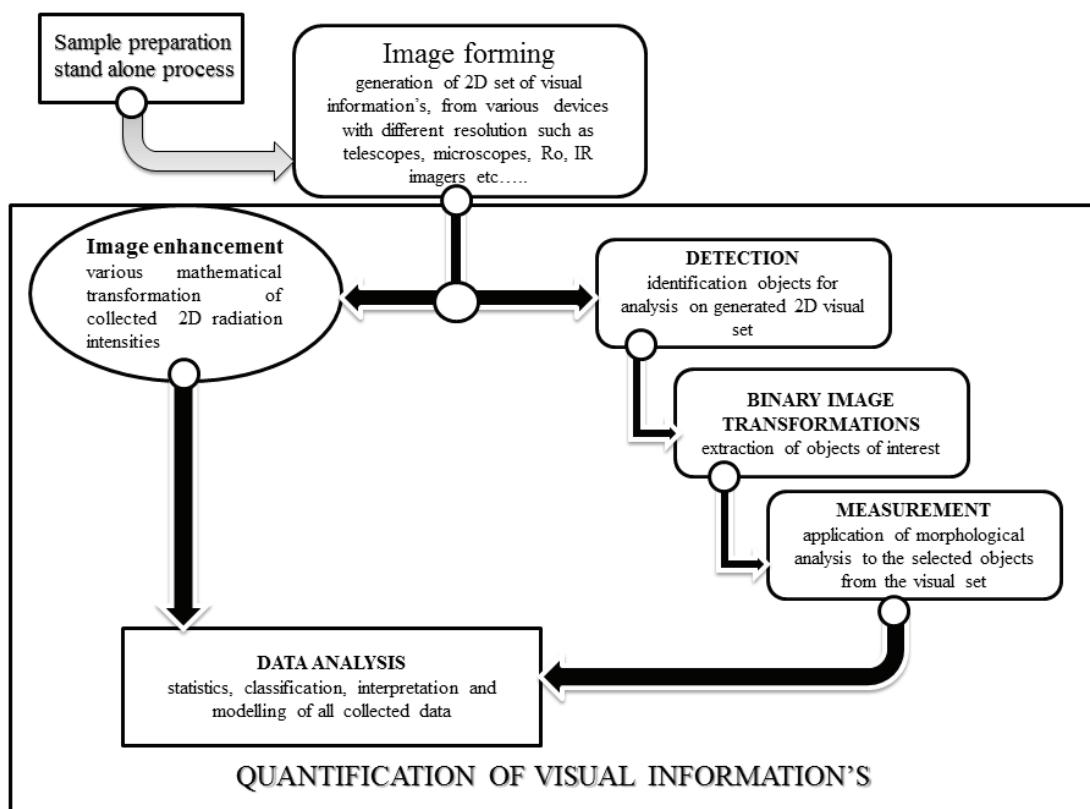
Figure 3. Schematic diagram of the quantification of visual information process.
