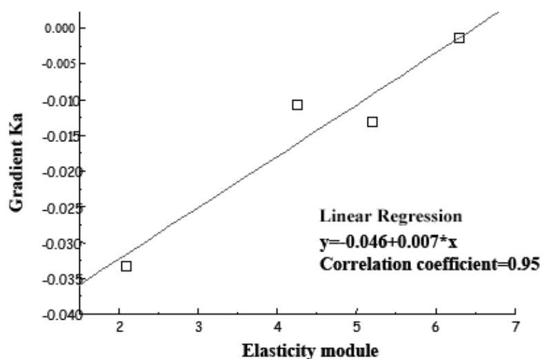
Figure 9. Regression analysis of the adhesiveness measurement results and mechanical characteristics of materials (y - gradient  $K_a$ , x - elasticity module).
