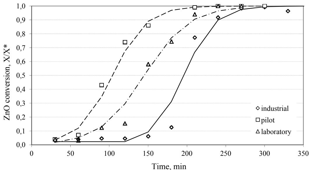
Figure 4. *ZnO Conversion vs. time graph of the experiments to observe the effect of scale-up (temperature 85 °C, seed amount 1.5%, initial reactants ratio ( $H_3BO_3$ :ZnO ratio of 5:1), and average particle size of zinc oxide particles of <1 µm were constant).*
