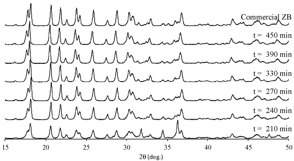
Figure 2. XRD Powder patterns of solid samples taken from the industrial scale experiment with respect to time (210–450 min) and commercial zinc borate Firebreak ZB.
