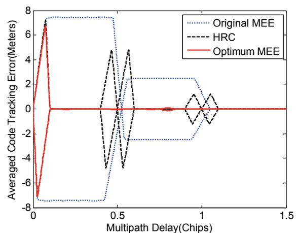
Fig. 5. MEE for original and optimum design and HRC (for BOC(1,1) signal).
