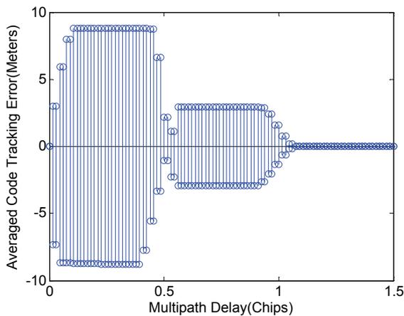
Fig. 2. The MEE of EML discriminator for BOC(1,1) signal. The multipath amplitude  $a_1=0.5$ ,  $\Delta=0.1$  chips.
