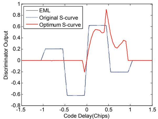
Fig. 4. The EML, original and the optimum S-curve (for BOC(1,1) signal).
