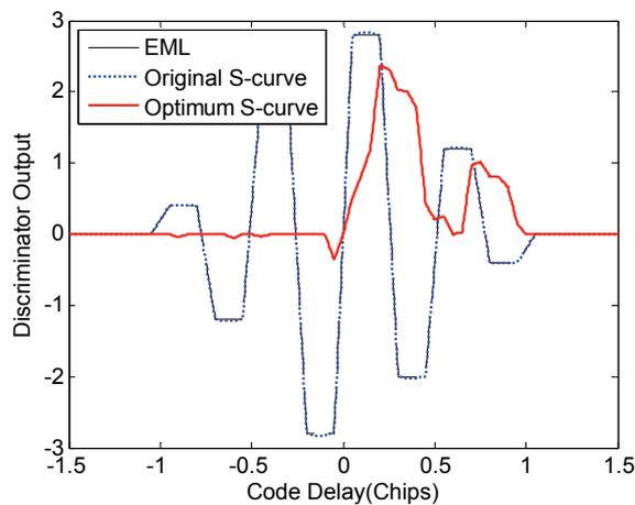
Fig. 7. The EML, original and the optimum S-curve (for BOC(10,5) signal).
