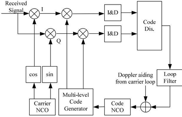
Fig. 1. Discriminator structure based on linear-combined code.
