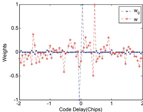
Fig. 3. The start point  $w_0$  and the optimum result  $w$  (for BOC(1,1) signal).
