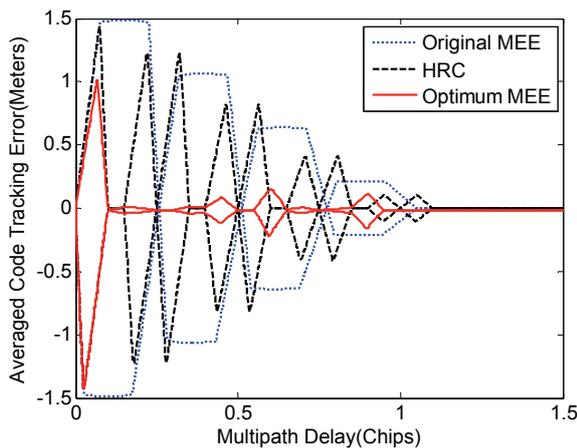
Fig. 8. MEE for original and optimum design and HRC (for BOC(10,5) signal).
