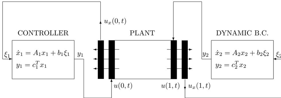
**Fig. 4.** The hybrid control system of the crane
