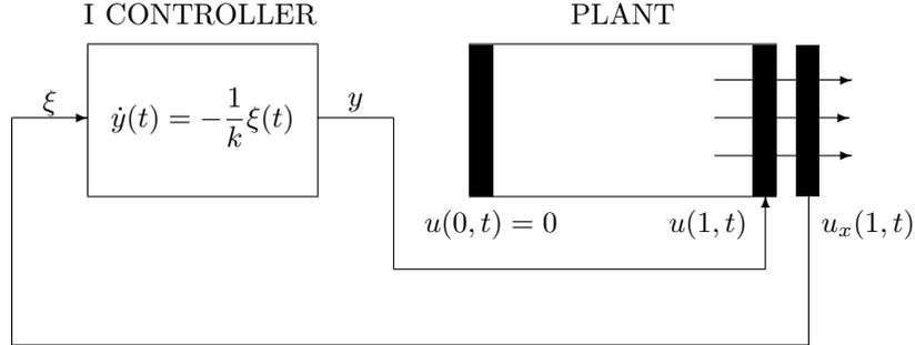
**Fig. 2.** Hybrid control system corresponding to (4.1)
