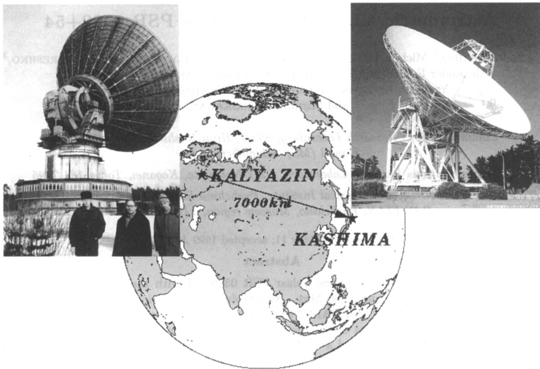
Fig. 1. Baseline of the Japan–Russia pulsar VLBI experiment. The Kashima 34-m diameter antenna of the CRL (upper right) and the Kalyazin 64-m diameter antenna of Moscow Power Engineering Institute (upper left) were used.
