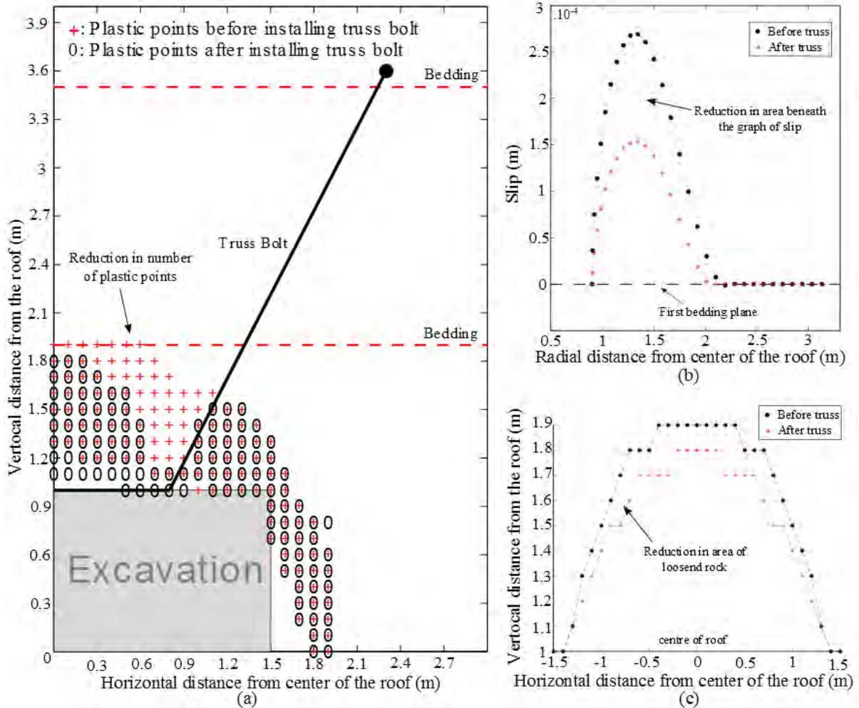
**Figure 2:** (a) plastic points distribution, (b) slip on the first bedding plane and (c) reinforced arch before and after installing truss bolt pattern ( $L=3\text{m}$ ,  $\alpha=60$ ,  $S=1.6$ ) on model 90250
