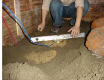
Figure 8: Burying of earth pressure cells
