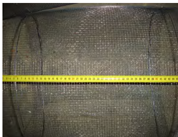
Figure 4: Wire mesh with \Phi 0.46@5\text{mm} Figure 5: Testing elastic modulus for test blocks
