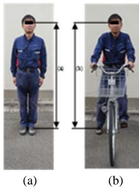
Fig. 12 Measured eye heights for a normal standing position (a) and a riding position on a bicycle (b).
