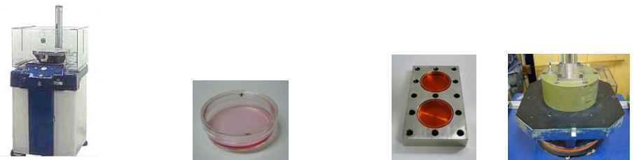
(b) Impact machine (c) Cultured dish and culture solution (d) Specimen container (e) Impact table
