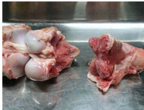
Fig. 4 Injury pattern of knee joint for drop height of 700 mm (test 1). Femoral epiphysis is fractured and the continuity of the epiphysis was completely destroyed.
