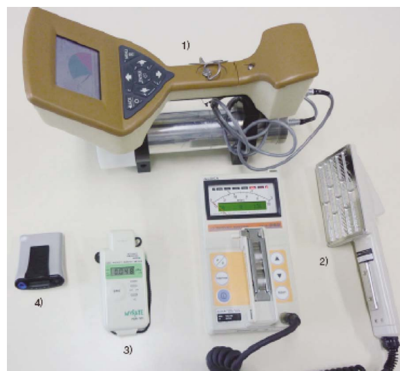
Fig. 1. (Color online) Portable laboratory. 1) gamma ray spectrometer 2inc NaI detector Mod1702 Ludlum Measurements Instruments Inc., 2) alpha and beta counter, TSC-362 Aloka, 3) dose rate meter, PDR-101, 4) dosimeter and dose rate meter, RAD-60S RADOS Technology.
