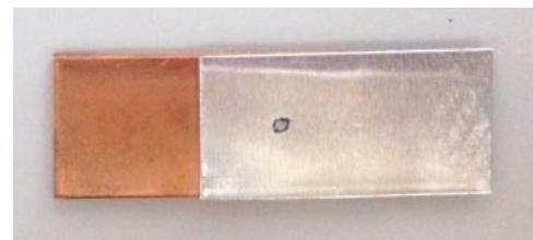
Fig. 11 Photograph of specimen. Vibration locus is the planar locus, and static pressure is 100 N.
