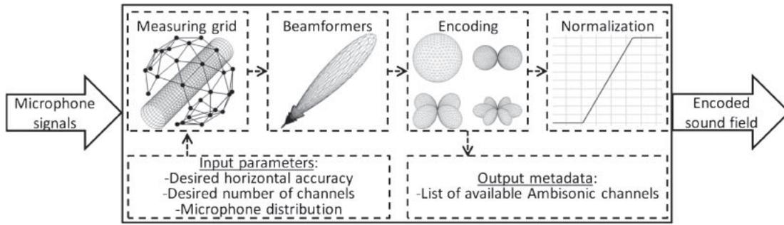
Fig. 3 Block diagram of the proposed mixed-order Ambisonics encoder for cylindrical microphone arrays.
