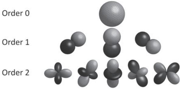
**Fig. 1** Spherical harmonic functions of order 0, 1 and 2. Bright lobes indicate positive values, dark ones are negative. There are  $2N + 1$  spherical harmonics of order  $N$ ; however, only two of them are needed to encode spatial information in the horizontal plane.
