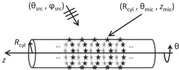
**Fig. 2** Layout of a cylindrical microphone array like those used by our proposal. The microphones are arranged as equispaced parallel rings on the surface of a rigid cylinder.
