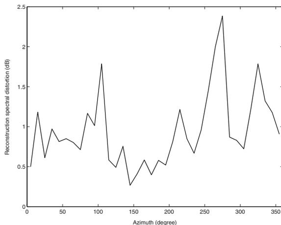
**Fig. 3** Reconstruction SD for each direction in the horizontal plane at the interpolation interval of  $10^\circ$ .
