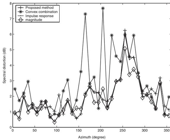
**Fig. 2** SD for each direction in the horizontal plane at the interpolation interval of  $10^\circ$ .
