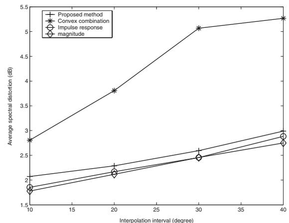
Fig. 1 Average SD across the horizontal plane as a function of interval angle.
