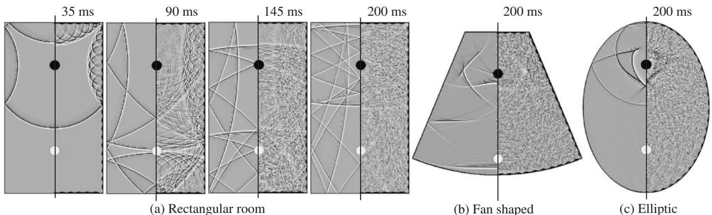
Fig. 6 Sound propagation visualized by FDTD methods in (a) rectangular, (b) fan-shaped and (c) elliptic rooms without (left-hand side) and with diffusing treatment (right-hand side).
