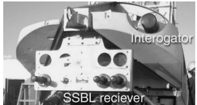
Fig. 3 Interrogator and SSBL receiver in the homing sonar.
