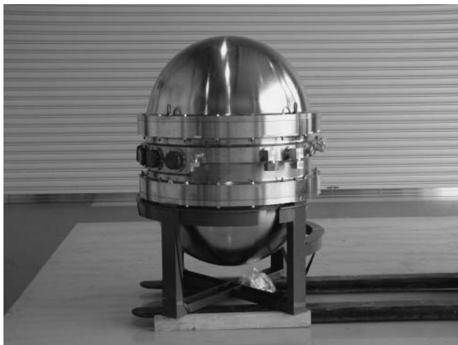
Fig. 12 Titanium alloy canister storing fuel cell stacks and equipment.
