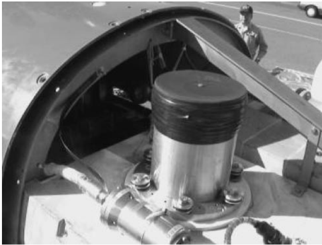
Fig. 6 Projector on the vehicle (for uplinks).
