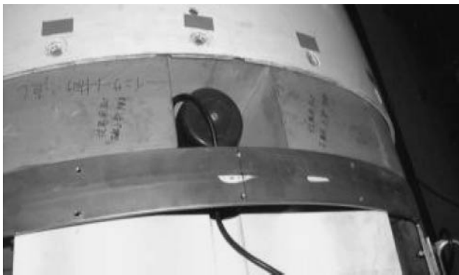
Fig. 7 Hydrophone on the vehicle (for downlinks).
