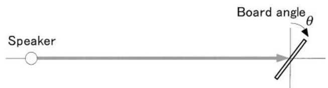
Fig. 3 Plan view of the setup to describe the board angle.
