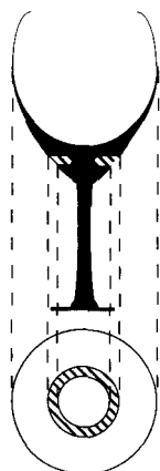
Fig. 7 Method for shaving a glass circumferentially.
