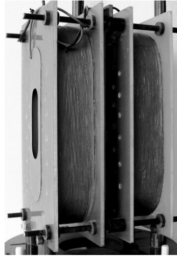
Fig. 5. Home-made race-track coils system.
