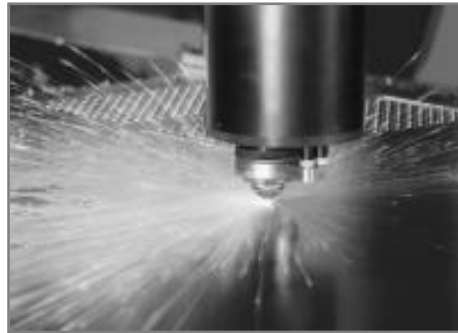
Fig. 3. Cutting bores with a laser cutter
