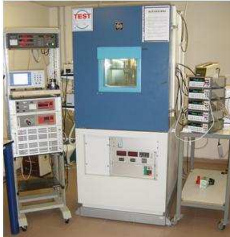
Fig. 4. The reference climatic chamber selected for the MID tests.
