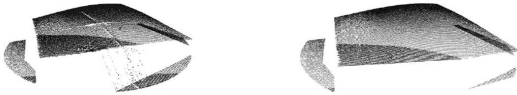
Fig. 6. Free form surface scanning result without (a) and with (b) the use of predictive algorithm.
