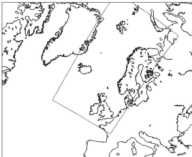
Fig. 1. Simulation area for storm surge model (small frame), inserted into simulation area of the regional atmosphere model and wave model. Northern corner of storm surge model area extends outside the area of atmospheric data. Here, data are extrapolated from nearest atmospheric data points, which have negligible influence on the results
