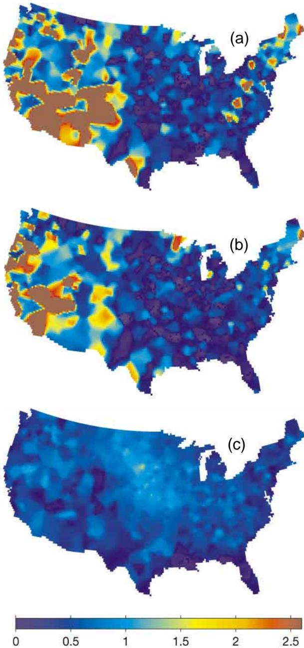
Fig. 7. Mean absolute error for 10-yr averages of July air temperature ( $^{\circ}\text{C}$ ) for (a) traditional spatial interpolation, (b) topographically aided interpolation, and (c) temporal substitution
