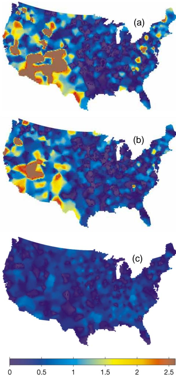
Fig. 5. Mean absolute error for 10-yr averages of annual air temperature ( $^{\circ}\text{C}$ ) for (a) traditional spatial interpolation, (b) topographically aided interpolation, and (c) temporal substitution
