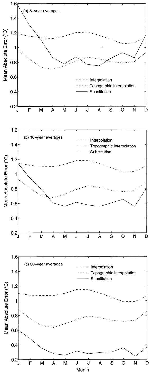
Fig. 8. Spatially averaged mean absolute errors of monthly air temperature ( $^{\circ}\text{C}$ ) for traditional spatial interpolation, topographically aided interpolation, and temporal substitution by month for (a) 5-yr, (b) 10-yr, and (c) 30-yr averaging periods. Note that the same scale is used for MAE on all 3 graphs
