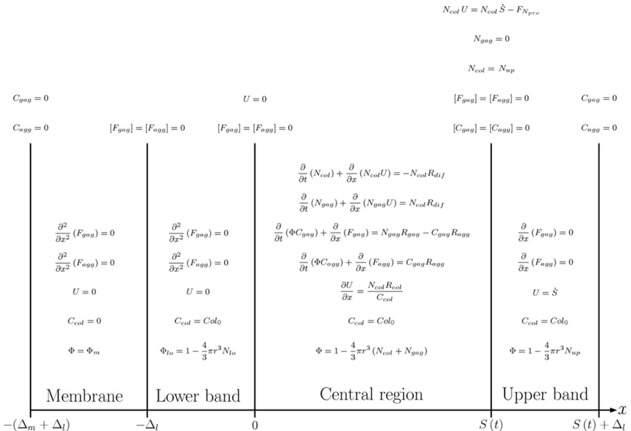
**Fig. 9:** Mathematical model of the four separate regions showing the relevant equations and continuity conditions between regions. Here the brackets [ ] represent the jump in the quantity across a boundary. The fluxes in each region are given by  $F_i = \Phi \left\{ C_i U - D_i \frac{\partial C_i}{\partial x} \right\}$ .
