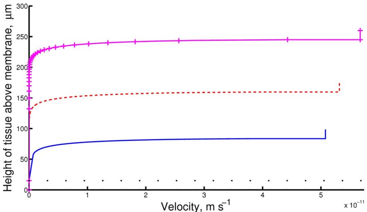
**Fig. 7:** The velocity of growth of the tissue layer, as predicted by the mathematical model, through the central region at 14 (—), 31 (- - -) and 49 d (—+—). Growth is a consequence of collagen production in this model, thus the only region that is expanding is close to the upper layer. The lower layer is denoted by a horizontal dotted line.
