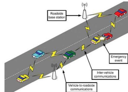
**Figure 1.3 Schematic Representation of a Vehicular Adhoc Network**
