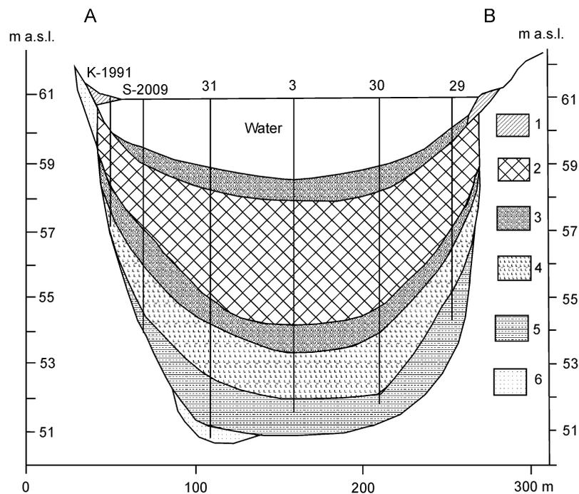
**Fig. 2.** Stratigraphy of Lake Prossa. For location of the cross section see Fig. 1B. 1, fen peat; 2, gyttja; 3, calcareous gyttja; 4, silt, in the upper part with plant remains; 5, laminated silt and varved clay; 6, sand.
