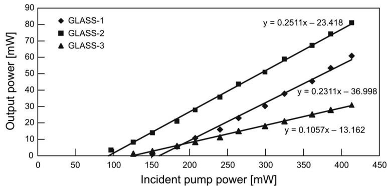
Fig. 5. Output power versus incident pump power of 974 nm wavelength for quasi-cw regime.
