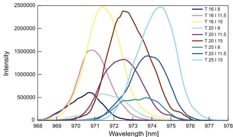
Fig. 2. Emission spectra of LIMO20-F100-DL976 laser diode.
