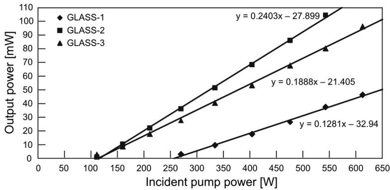
Fig. 8. Output power versus incident pump power of 939 nm wavelength for cw regime.
