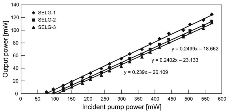
Fig. 9. Output power versus incident pump power of 974 nm wavelength for quasi-cw regime.
