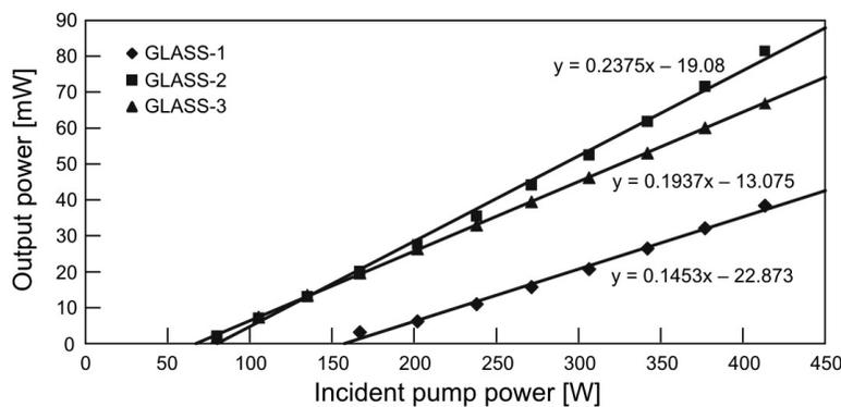
Fig. 6. Output power versus incident pump power of 974 nm wavelength for cw regime.
