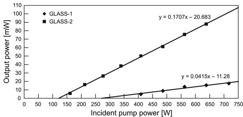
Fig. 13. Output power versus incident pump power of 939 nm wavelength for cw regime without optics.
