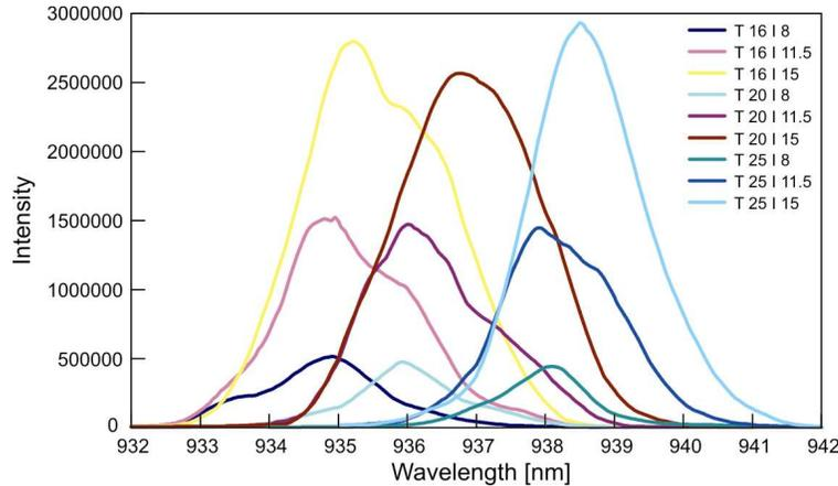
Fig. 3. Emission spectra of LIMO20-F100-DL940 laser diode.
