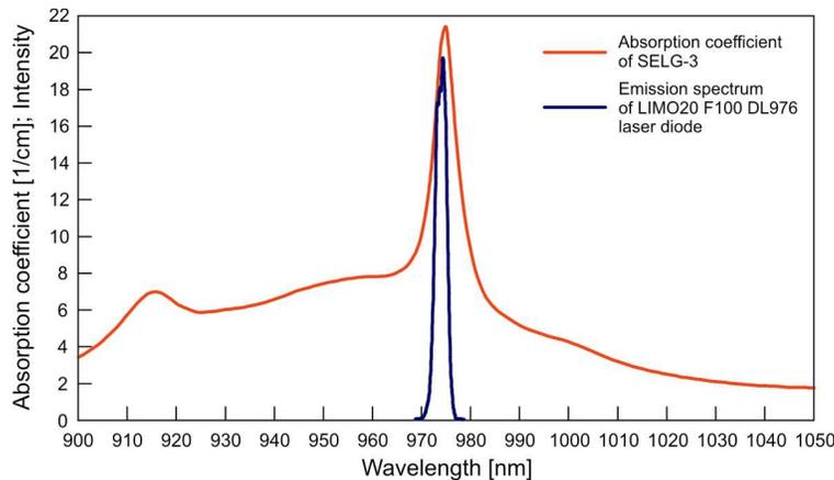
Fig. 4. Emission band of LIMO20-F100-DL976 laser diode at temperature 27 °C on the background of absorption coefficient of SELG-3 sample.
