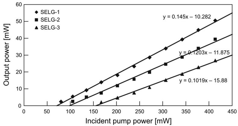
Fig. 11. Output power versus incident pump power of 939 nm wavelength for quasi-cw regime.
