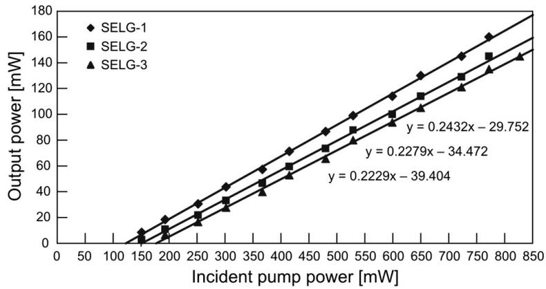
Fig. 10. Output power versus incident pump power of 974 nm wavelength for cw regime.
