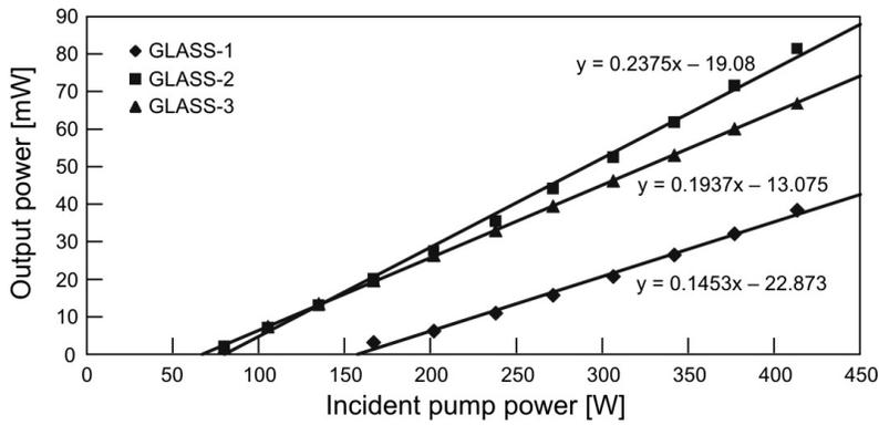
Fig. 7. Output power versus incident pump power of 939 nm wavelength for quasi-cw regime.
