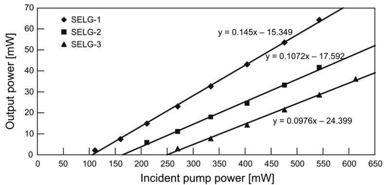
Fig. 12. Output power versus incident pump power of 939 nm wavelength for cw regime.
