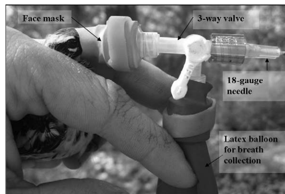
FIG. 1. Sampling unit used to collect breath samples from migrant landbirds as described in Hatch et al. (2002a). The breath sampling unit was composed of a three-way stopcock valve, face mask, and balloon collection chamber. The balloon was flushed and filled with pure oxygen, which the bird was allowed to breathe for 20 s. Collected CO 2 was immediately transferred to an evacuated Exetainer tube for future stable-carbon-isotope analysis.
