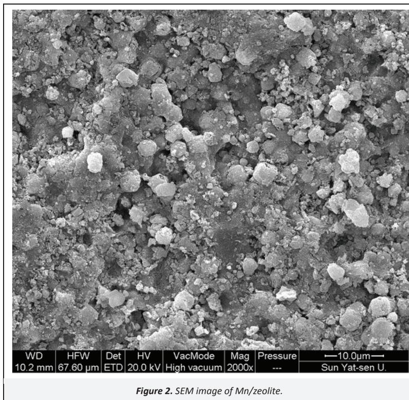
Figure 2. SEM image of Mn/zeolite.
