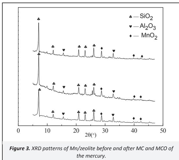
Figure 3. XRD patterns of Mn/zeolite before and after MC and MCO of the mercury.
