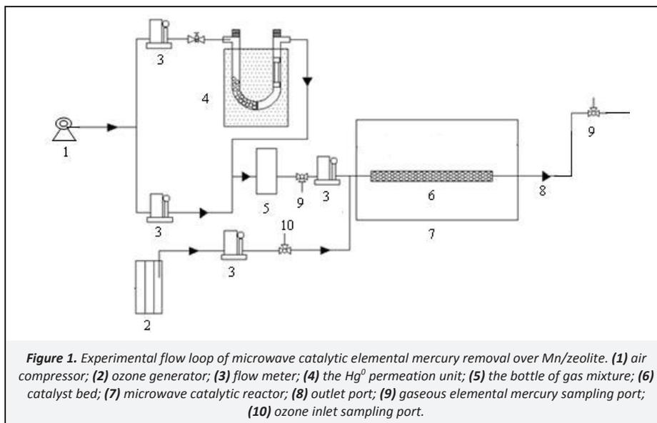
**Figure 1.** Experimental flow loop of microwave catalytic elemental mercury removal over Mn/zeolite. (1) air compressor; (2) ozone generator; (3) flow meter; (4) the Hg<sup>0</sup> permeation unit; (5) the bottle of gas mixture; (6) catalyst bed; (7) microwave catalytic reactor; (8) outlet port; (9) gaseous elemental mercury sampling port; (10) ozone inlet sampling port.
