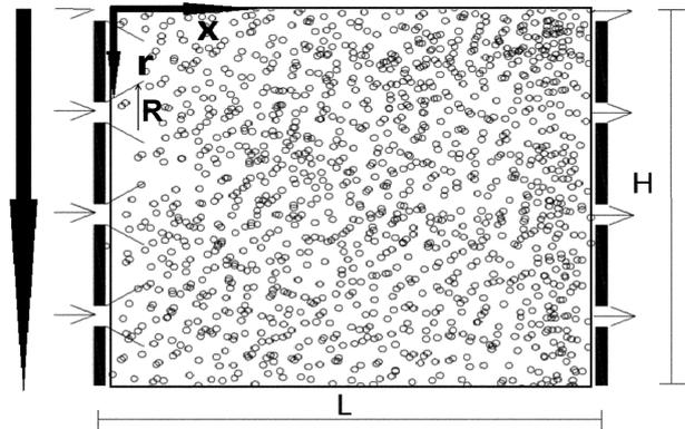
Fig. 1. Scheme of the particles dryer.  $R$  – jet radius,  $L$  – hopper width,  $x$  – axial direction of the jets,  $r$  – radial coordinate.
