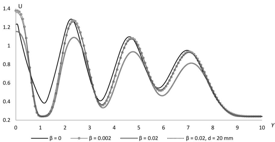
Fig. 8. Distribution of the axial gas velocity  $U$  at  $X = 9.9286$  for different particles volume fractions.
