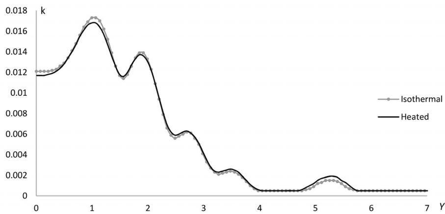
Fig. 7. Distribution of the turbulent kinetic energy  $k$  at  $X = 19.9286$  for the isothermal and heated cases.
