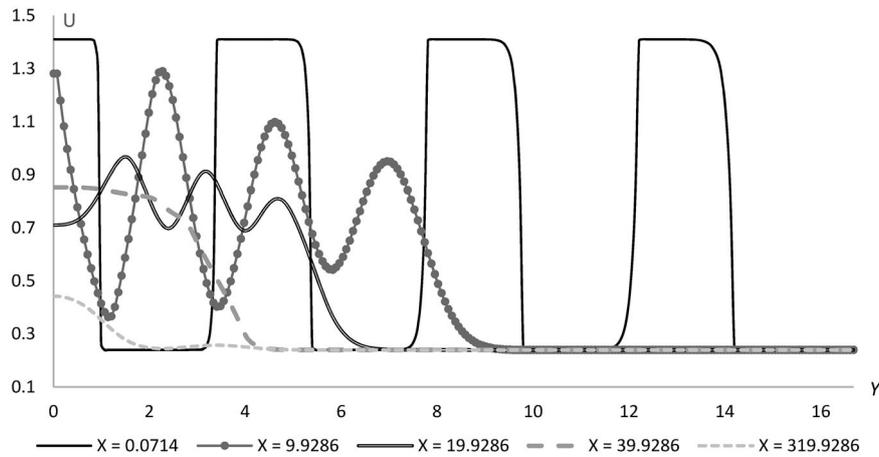
Fig. 2. Distribution and evolution of the axial gas velocity  $U$  for the isothermal case.
