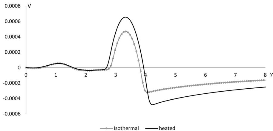
**Fig. 5.** Distribution of the radial gas velocity  $V$  at  $X = 39.9286$  for the isothermal and heated cases.
