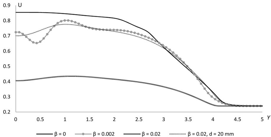
Fig. 9. Distributions of the axial gas velocity  $U$  at  $X = 39.9286$  for different particles volume fractions.
