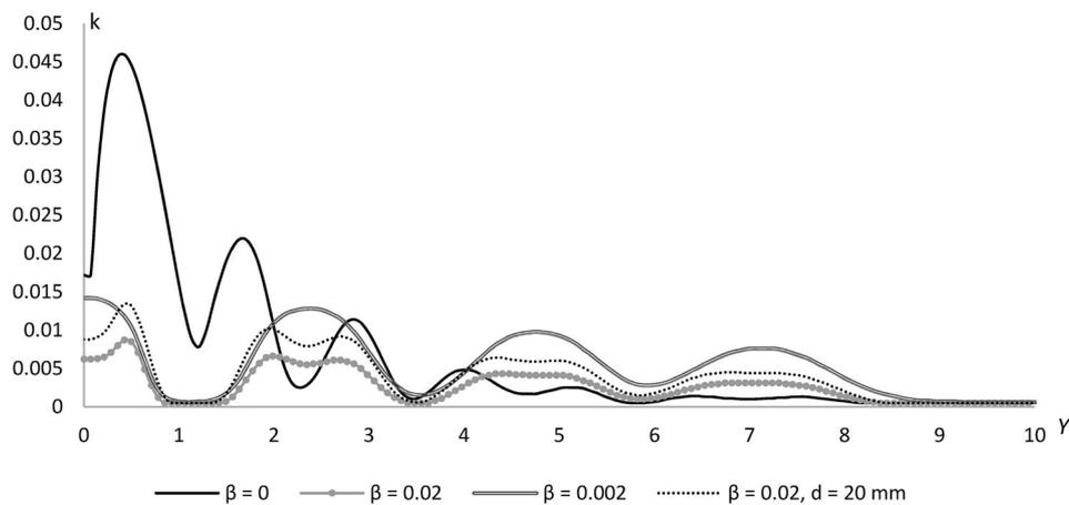
Fig. 13. Distribution of the turbulent kinetic energy  $k$  at  $X = 9.9286$  for different particles volume fractions  $\beta$ .
