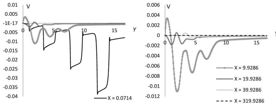
**Fig. 4.** Distribution and evolution of the radial gas velocity  $V$  for the heated case with (a)  $X = 0.0714$  and (b) without it.
