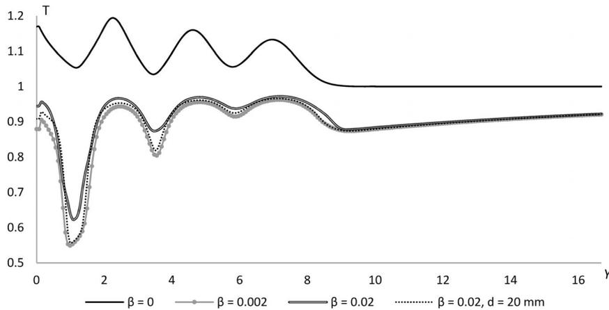
Fig. 11. Distributions of the temperature  $T$  at  $X = 9.9286$  for different particles volume fractions  $\beta$ .
