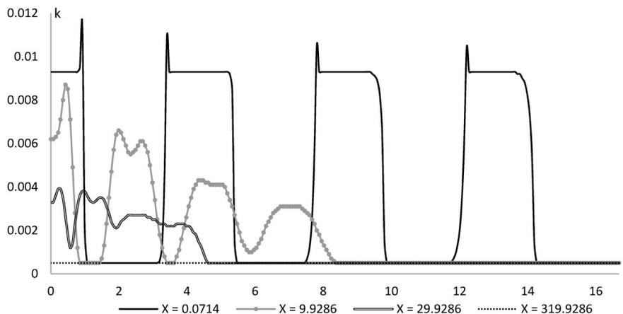
Fig. 12. Evolution of the turbulent kinetic energy  $k$  for the case of particles volume fraction  $\beta = 0.002$ .
