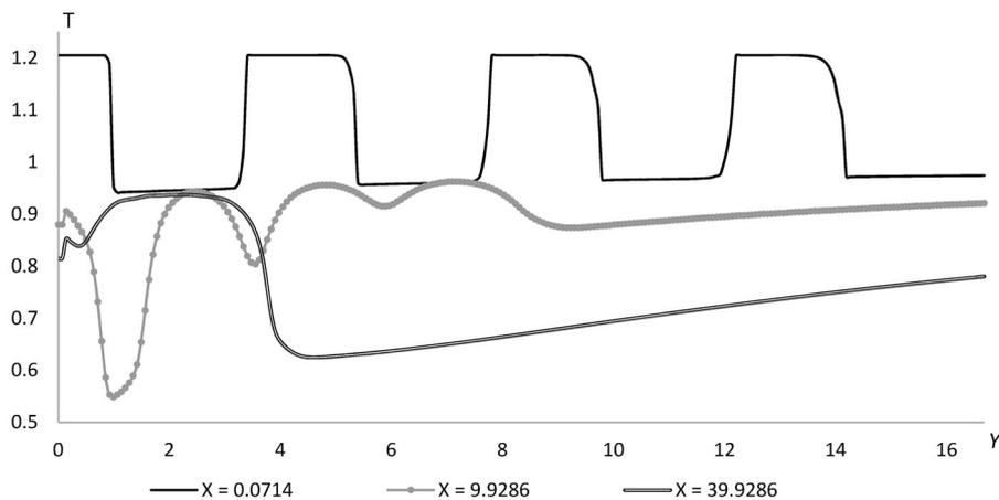
Fig. 10. Evolution of the temperature  $T$  for the case of particles volume fraction  $\beta = 0.002$ .
