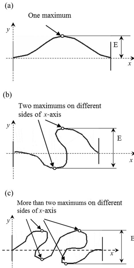
**Fig. 4.** Types of shapes of waves: a – Type 1, b – Type 2, c – Type 3. E – height of wave.
