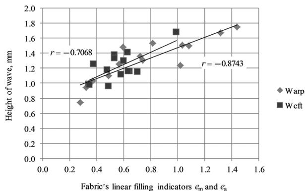
Fig. 6. Relationship between the height of the wave and linear filling indicators of the fabric  $e_m$  and  $e_a$ .
