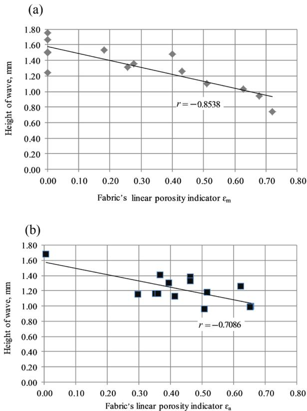
Fig. 5. Relationship between the height of the wave and the fabric's linear porosity indicators: (a) in the warp direction, (b) in the weft direction.
