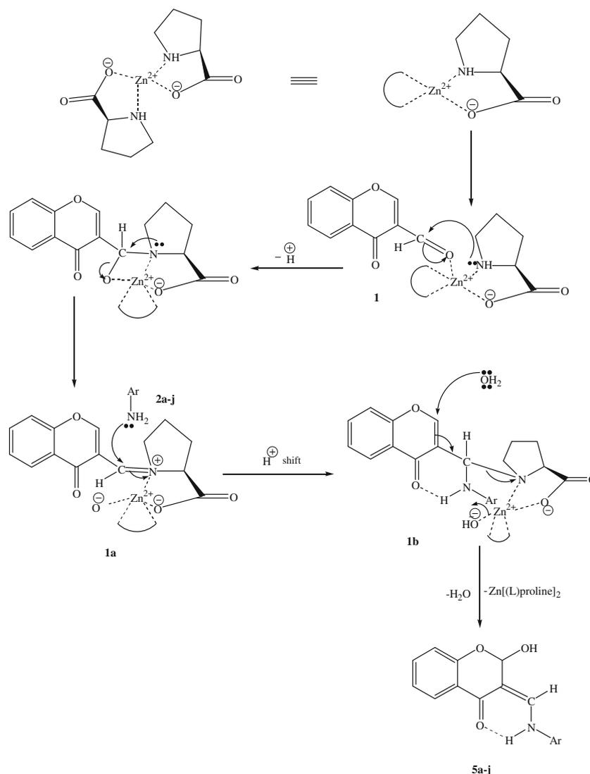
**Scheme 3.** Proposed mechanism for the Zn[(L)proline]<sub>2</sub> complex catalysed synthesis of chromanone derivatives (**5a–j**).
