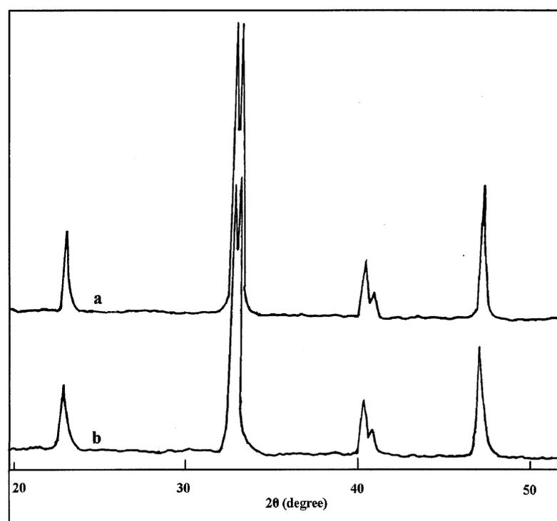
**Figure 4.** XRD spectra of LaMnO<sub>3</sub> [without treatment (a), treated with water at 225°C (b)].
