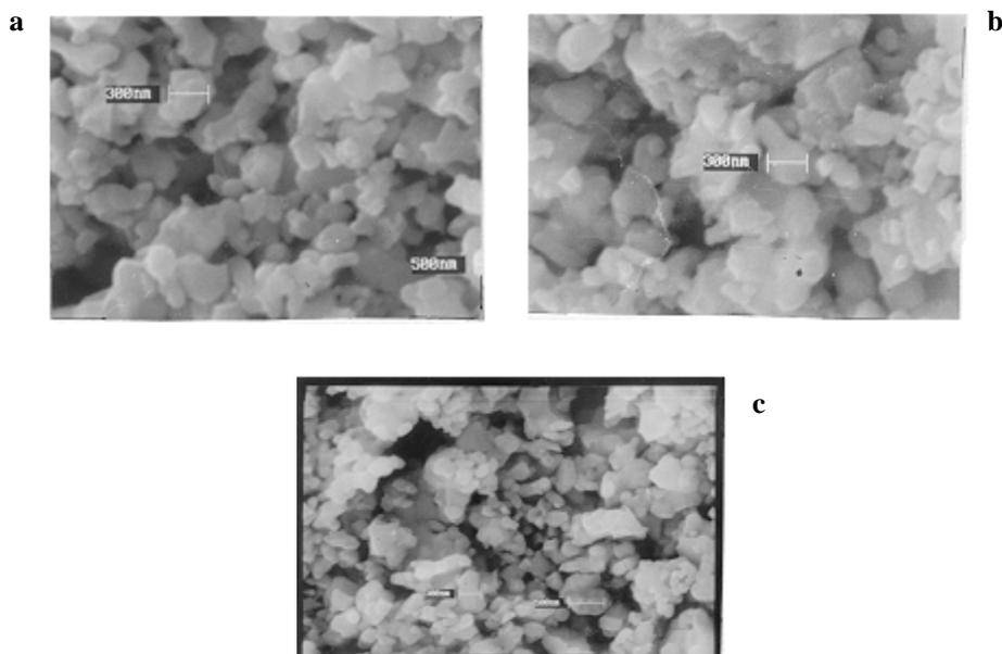
**Figure 2.** Scanning electron micrograph of  $\text{LaMnO}_3$  without water treatment (a), treated with water at  $225^\circ\text{C}$  (b) and at  $300^\circ\text{C}$  (c).
