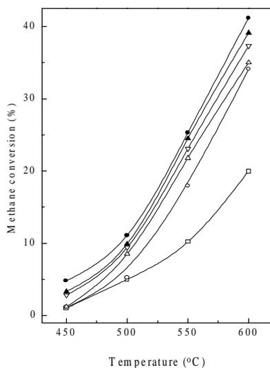
**Figure 6.** Effect of temperature on the conversion of methane in its complete combustion over  $\text{LaCoO}_3$  – treated with steam at  $350^\circ\text{C}$  (○),  $500^\circ\text{C}$  (△),  $600^\circ\text{C}$  (▽),  $700^\circ\text{C}$  (▲),  $800^\circ\text{C}$  (●) and without water treatment (□).
